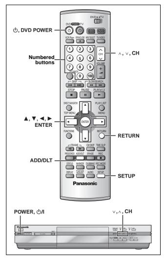
After plugging the unit into your household AC outlet and pressing [ $\dot{\oplus}$ , **DVD POWER**] to turn the unit on for the first time, the unit assists you to set the menu language, and automatically tunes in all the channels it can receive and sets the clock.
